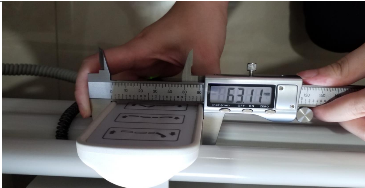
Figure 3. Rehabilitation engineer engaged in the process of measuring the dimensions of an electric bed remote control.
