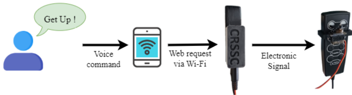
Figure 2. Working Mechanism of Bedriod System. Patient speaks the preset voice command to smart device, and the smart device recognizes the command and activates the built-in voice assistance function. Smart device sends the corresponding web request to Bedriod system via the local Wi-Fi environment. The Bedriod system then fires electronic signal to servo motor for pressing the corresponding button on eclectic bed remote control.
