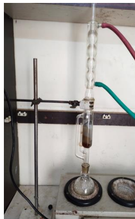
Fig 6 Soxhlet extraction apparatus used for extraction process.
