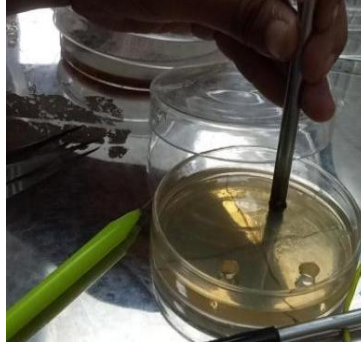
Fig8.2:- Well Method by cork borer
