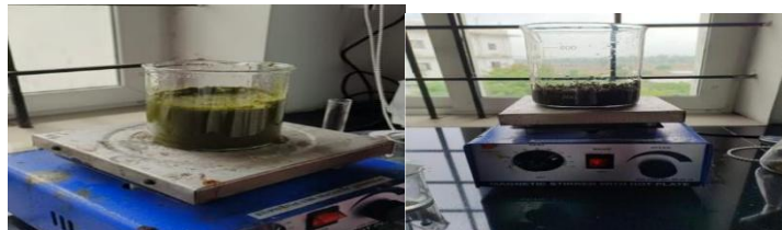
Fig (a): Extract formation of Amla leaf Fig(b):Extract formation of Adua leaf Fig 3:-Leaf extract formation by using Magnetic stirrer
