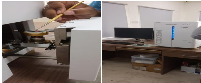
Fig12.6:- Amla and adusa based AgNPs Sample loading on SEM
